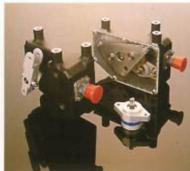
Aircraft flap and position feedback potentiometers
