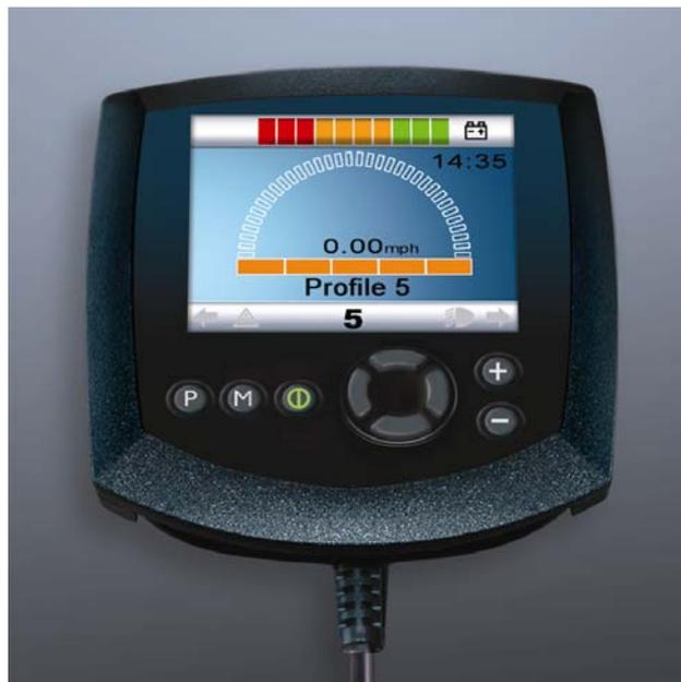
The R-net Omni features a large, full color LCD screen with real-time clock and speedometer, housed in a compact and ergonomic package. Much consideration has been given to the screen layouts, to ensure they present the user information in the clearest and most user-friendly way. In addition, the content and order of user menus is fully customizable, a feature that ensures the most frequently used and popular functions can be accessed in the most efficient way.
