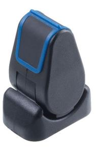
The JC1210 builds on the success of the JC1200, incorporates the same robust design with exceptional life, and now offers the option of overpress and latch features at the ends of travel. This new joystick utilizes non-contacting, Hall-effect sensing technology for long-life integrity of the output signal. Operating feel has been an important part of this new development to make this unit as smooth and easy to operate as possible throughout a 5 million cycle life to the start of overpress
