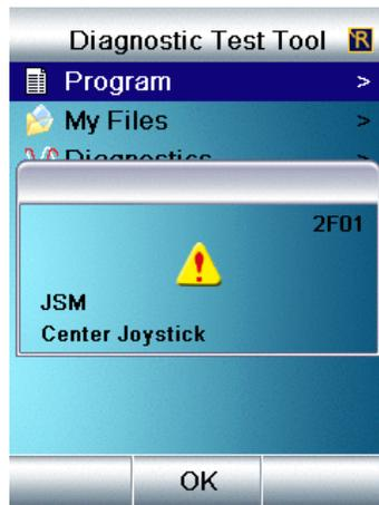
If the powerchair is suffering from intermittent errors, then the DTT can be used to inspect each of the R-net modules' system logs in order to build up a history of what may have been happening. Taking this one stage further, the log files can also be transferred to a PC and emailed back to a technical center for detailed analysis.
