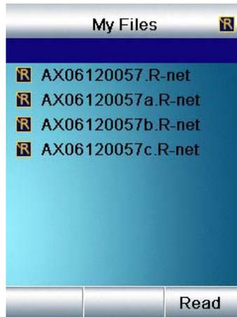
If a memory stick is connected, then files can be saved directly onto the stick itself. Navigating to the Memory Stick folder and then exercising the Read command achieve this. When the DTT is connected to a PC, then it will appear as a conventional drive with the name DTT and conventional Windows® commands can then be used to organize folders and files, including Rename, Copy and Delete options.
