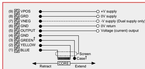
Misconnection of the supply may cause permanent damage
