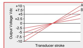
Note: A and B outputs only available with a  $\pm(13.5 - 30)$  Vdc supply
