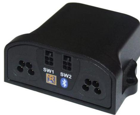
The iDevice Module enables the wheelchair user to control their iPad, iPod or iPhone using any R-net Input device e.g. a Joystick Module or an Omni. Deflecting the joystick forward, backwards, left and right navigates and select icons or menu items. The set-up procedure is intuitive and no specialist software is required to be installed on the iDevice.
