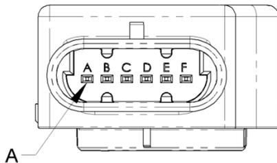
Mating connector type: Packard Electric 'Metri-Pack' 150 series or equivalent
