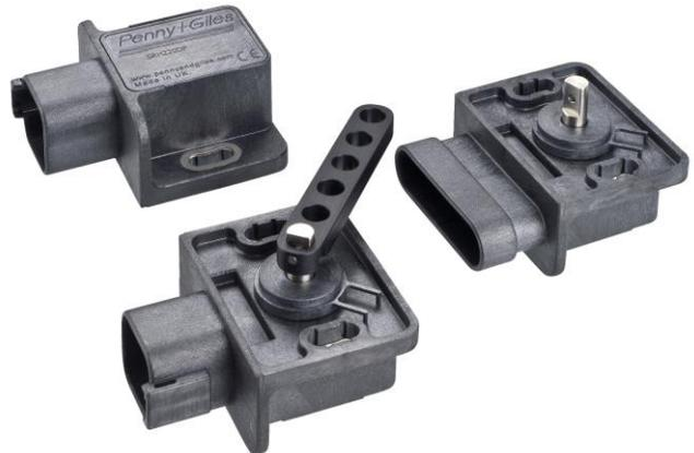
The SRH220DR is a shaft-operated, No Contact rotary position sensor with dual-redundant outputs. The versatile, factory-programmable electronics, which can be supplied from 5V or 9-30V, can be easily set to one of three analog voltage output ranges or one of three PWM frequencies. In addition, the polarities of the analog outputs can be set to one of three combinations – both tracking in the same direction or one opposite to the other.
