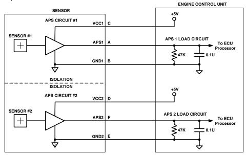
To aid with ECU diagnostic functions, this sensor is specified to output predetermined voltages in the event that power supply lines or the ground lines are broken. The ranges for these voltages is specified in the 'Electrical Specifications' table under the parameter  $V_{\text{DIAG}}$ . This voltage is specified for a number of fault and loading conditions.
